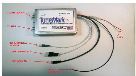
1) 12v power leads: These leads can be paralleled with radio power if desired, as they draw no current until TuneMatic is powered up by Radio Control cable. **NEGATIVE GROUND SYSTEM ONLY!**
